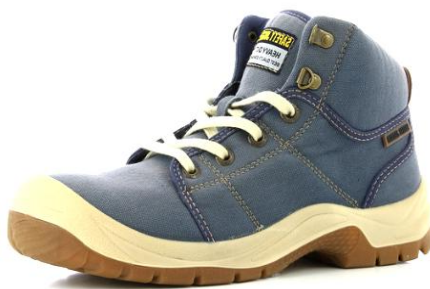
Item No.: 86120 Upper: Canvas Outsole: Dual Density PU Midsole: Kevlar Plate Toe: EN Standard Steel Toe Safety Standard: S1p
