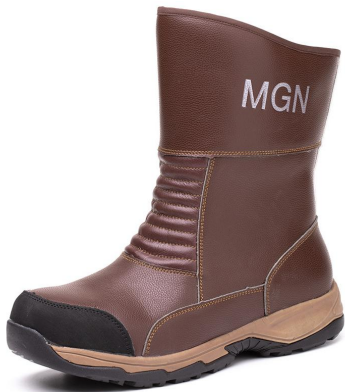
Item No.: 1616 Upper: Microfiber Leather Outsole: MD Rubber Midsole: Steel Plate Toe: EN Standard Steel Toe Safety Standard: S1p
