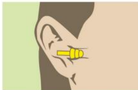
Insert the earplug so all flanges are well inside your ear canal.
