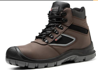
Item No.: 1413 Upper: Microfiber Leather Outsole: Dual Density PU Midsole: Kevlar Plate Toe: EN Standard Steel Toe Safety Standard: S1p
